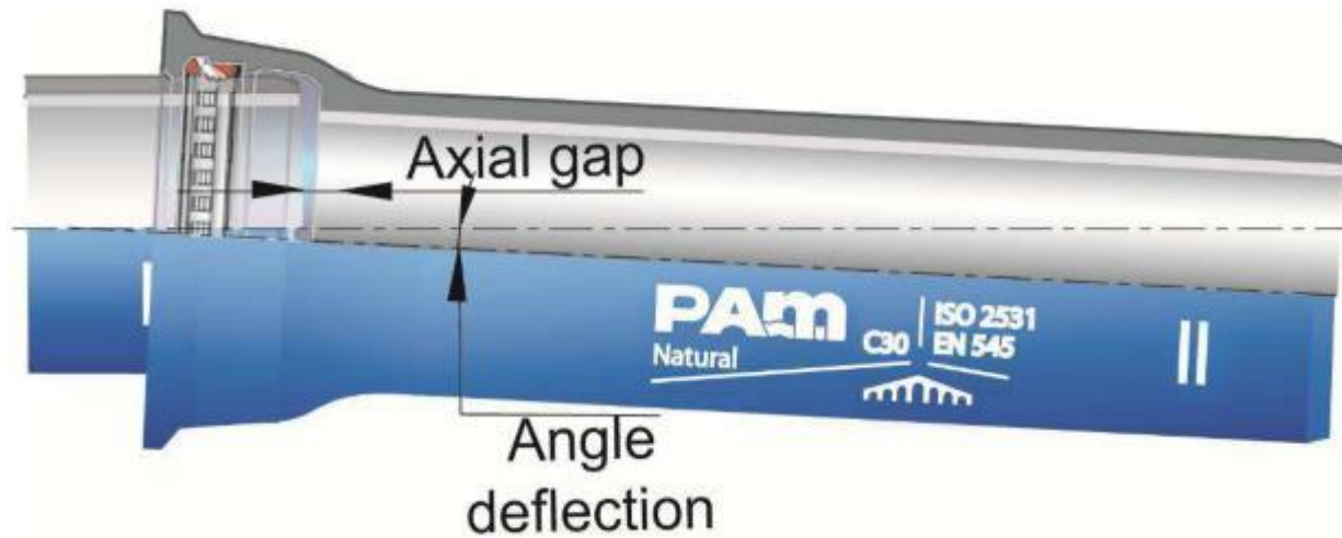
Figure 4. 4: Standard Vi Joint for pipes
